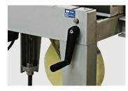
EASY CASE SIZE CHANGES Tool-less case size changes are simple and quick with change points accessible from both operational sides of the machine.
