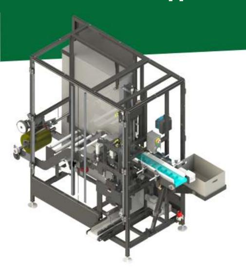
The **AF-20 Potato Wrapper** uses our patented belt design to wrap potatoes in aluminum foil. This one-of-a-kind machine uses rolls of foil instead of individual sheets. Product is brought in and dropped softly into catch gates. A photo eye triggers the plunger to gently drive the product through the precut foil and into the wrapping belts. The wrapped product is deposited onto the discharge conveyor.
