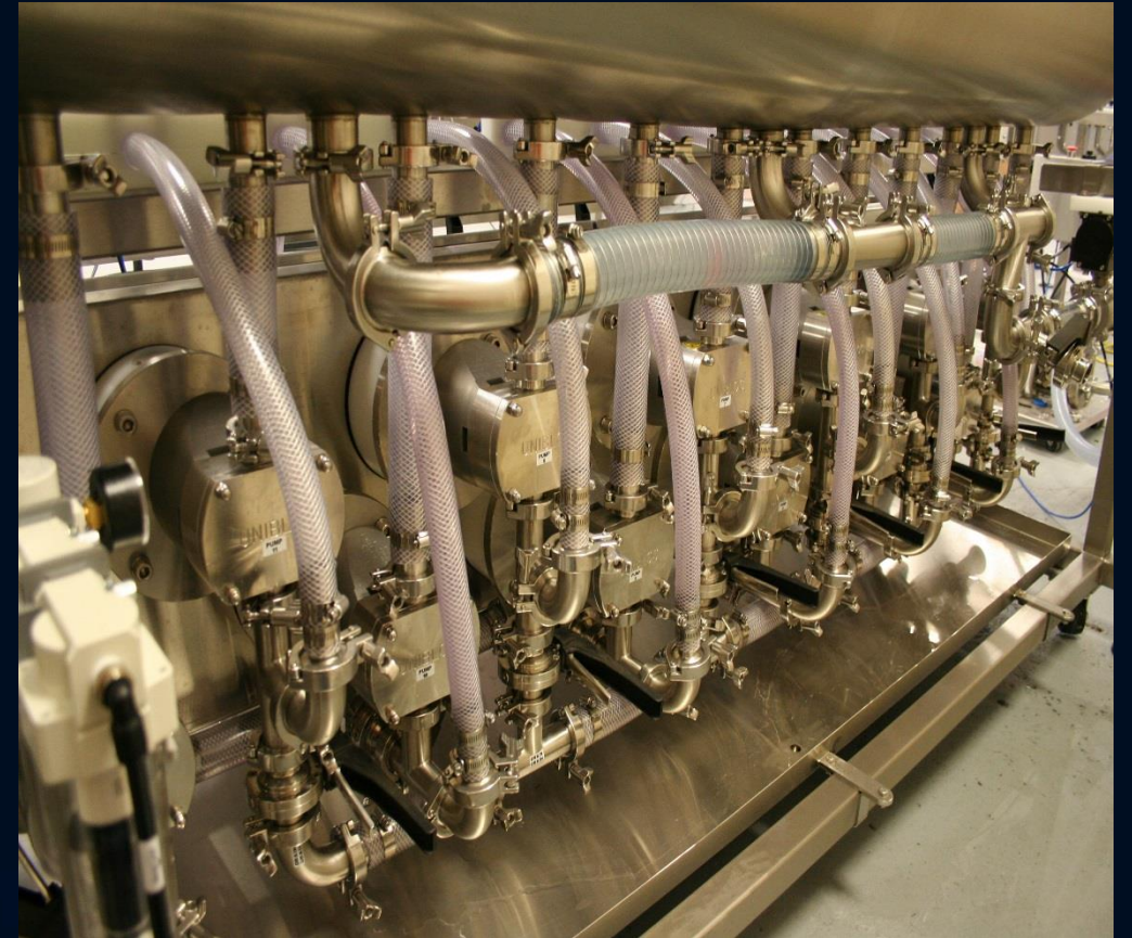
Each nozzle has an application specific pump and drive system
