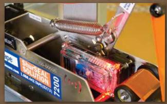
Operators have more control on the packaging line, with the ability to immediately address case sealing issues. Prime-Alert offers visual and audible alerts to signal five case sealing issues: low tape, no tape, broken tape, uncut tape and case jams.
