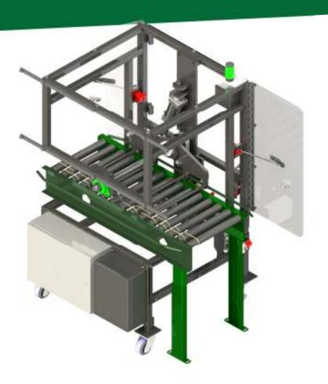
The **Case Flipper System** was designed and built to flip sealed cases to the proper orientation, for the next machine in the production line. It should be used on Automated Packaging Lines that utilize existing live roller style conveyors. This system is able to be pulled in/out of service rapidly.
