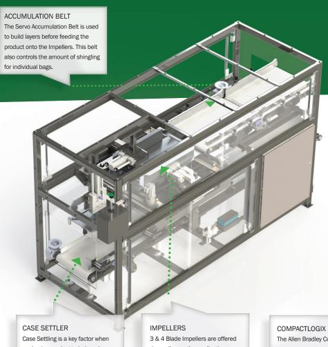
Case Settling is a key factor when packaging product to help reduce head space in the case. The capability to settle each layer as it's placed in the case also ensures maximum settling capabilities.
