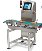
There are multiple approaches to supplying feedback information. One way is to provide weight information on a per-package basis. The production line's PLC can take that data and trigger whatever action is necessary to keep the fill within the appropriate range.
