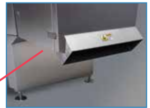
Good product outfeed chute (rejects drop down to bin or takeaway conveyor)
