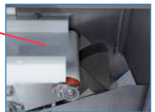
Multilane rejection gates (other rejecters available for small products)
